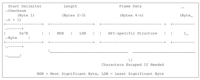
When sending or receiving an API2 frame, specific data values must be escaped (flagged) so they do not interfere with the data frame sequencing. To escape an interfering data byte, the byte 0x7D is inserted before the byte to be escaped XOR'd with 0x20.
