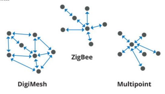
**Note:** Not all XBee devices can run all these communication protocols. The combination of XBee hardware and radio firmware determines the protocol that an XBee device can execute. Refer to the XBee RF Family Comparison Matrix for more information about the available XBee RF modules and the protocols they support.
